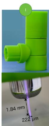
Fig 2. A) Final design of a 3D printed LTP probe. B) Spatial dimensions of the LTP [3].
