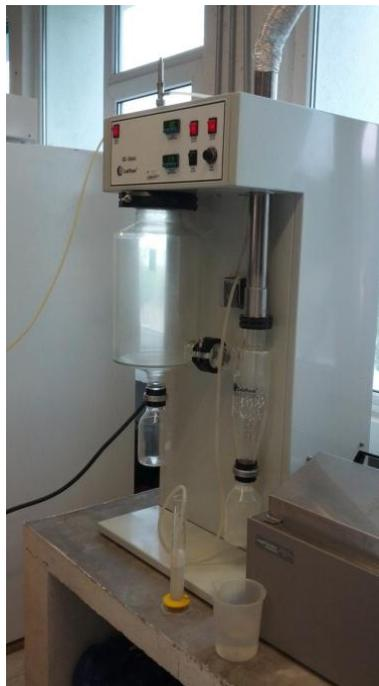
Figura 5.1.2 Spray dryer SD-Basic.
