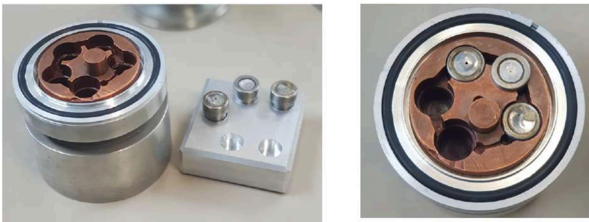
Figure 12. The vacuum connector 63 ISO, on which is based the copper block that receive the Knudsen effusion cells used.
