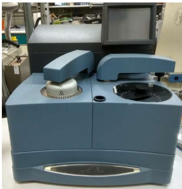
Figure 9. Differential Scanning Calorimetry (DSC) Q2000 device used to perform the purity, temperature and enthalpy of fusion experiments.
