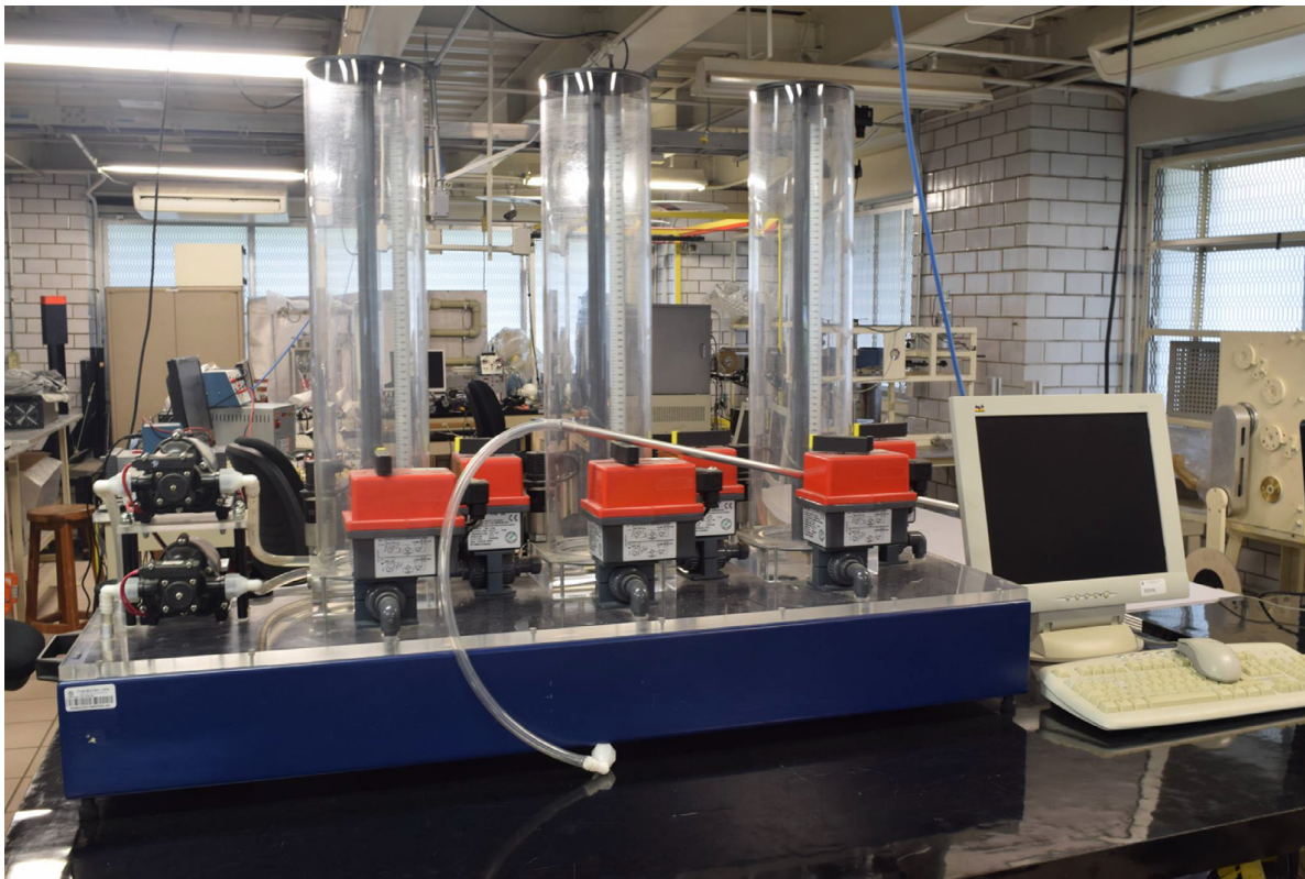
Fig. 9. Amira DTS200 three-tank system benchmark.
