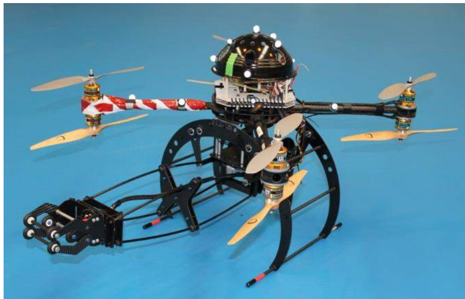
FIGURE 1.1: Aerial 6 DoF manipulator proposed by the ARCAS project
