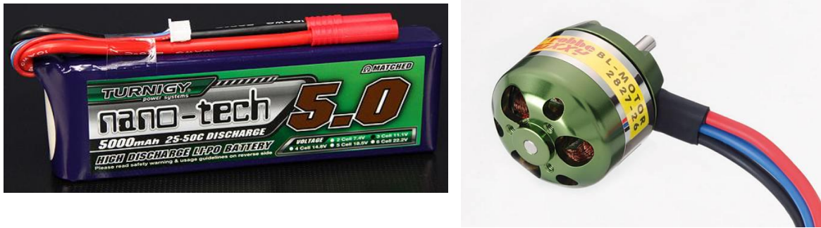
Fig. 3.4: LiPo battery and brushless motor.
