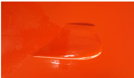
(c) Pylon with Tooling Gel Coat
