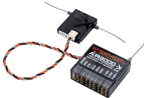
Figura 2.16: Receptor SPECKTRUM AR8000
