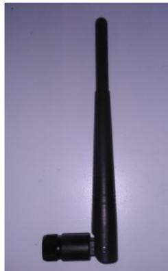
Figura 3.9: Antena dipolo *GW.59*
