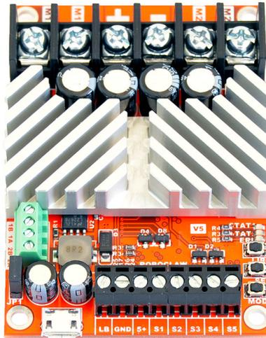
Figura C.4: Driver RoboClaw ST 2X45A.
