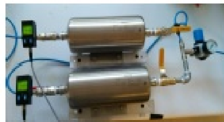
Fig. 6. Tanks of compressed air that contains 4 liters to 10 bar for the supply of energy in the pneumatic actuators.
