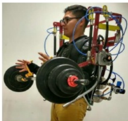
Fig. 1. Force augmenting hybrid exoskeleton for the elbow joints.
