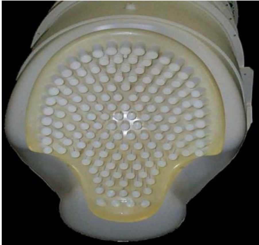
Figure 3 The 151-sensor array of the SARA system.
