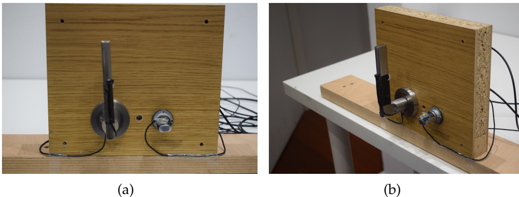
Figure 3.2: Wooden board simulating a door, used in the experiment. (a) Door lever handle and a door lock handle. (b) Photodiode and push bottom instrumentation to detect each grasp time.
