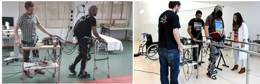
Figure 1.4: Control of an ambulatory exoskeleton with a Brain Computer Interface for spinal cord injury gait rehabilitation [37]
