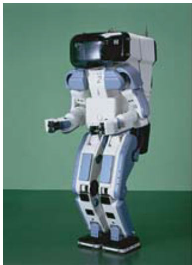
(a) Honda P2 (180 cm de altura, 210 kg) [2]
