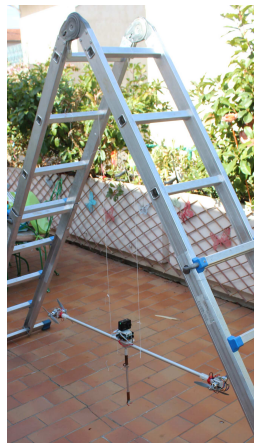
Figure 1.13: bench test rotational inertia measure
