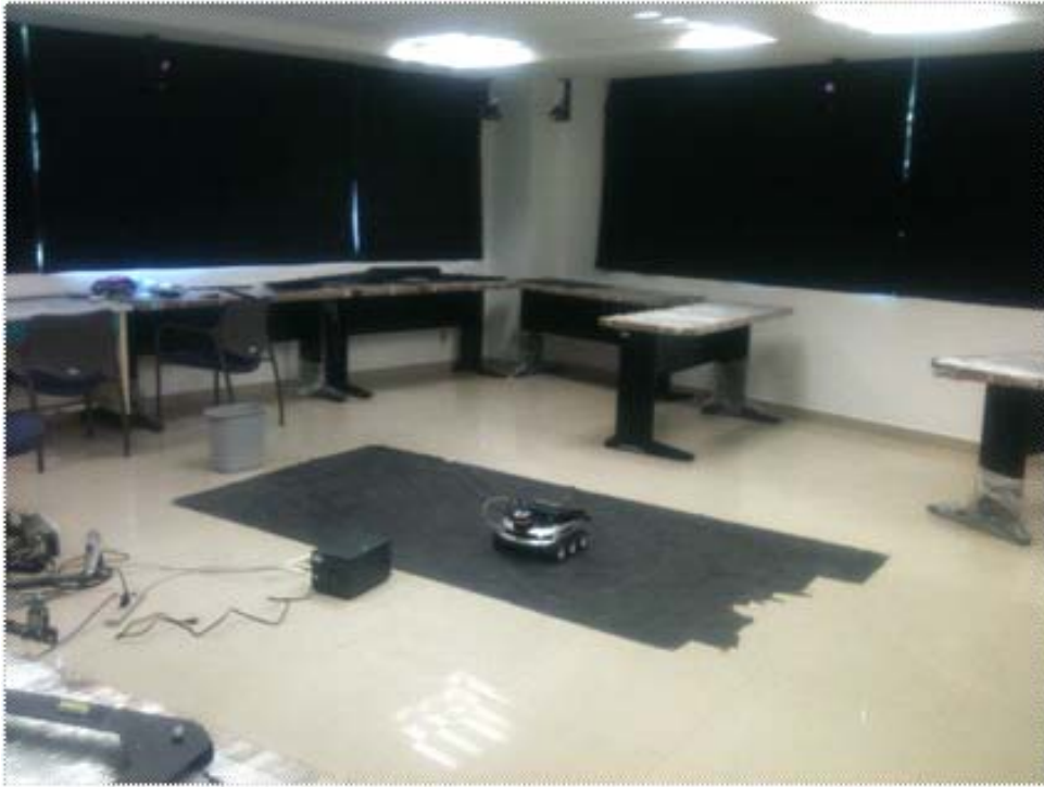
Figure 3.9: The experiment in an office environment equipped a motion capture system
