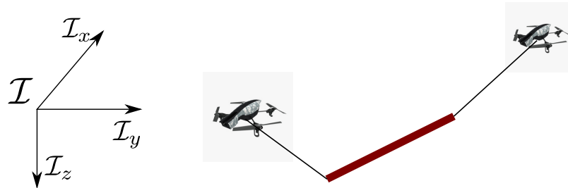
Figure 5-1: Slung-load configuration of the two quadcopters cooperatively carrying a bar. The inertial frame \mathcal{I} can be separated into two perpendicular planes x - z and y - z .
