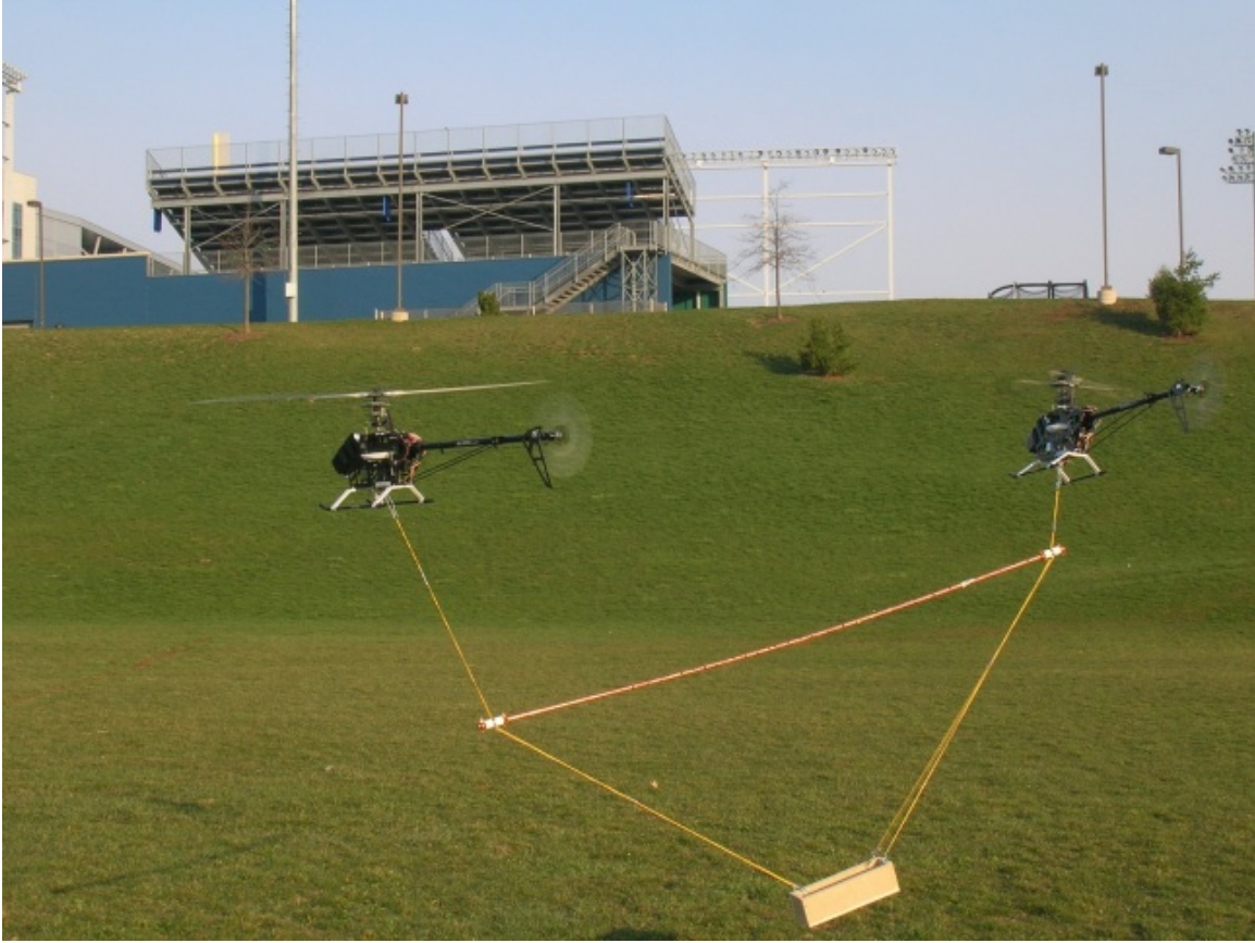
Figure 1-5: An example of a cooperative scheme to transport a load using a cable mechanism with a bar.
