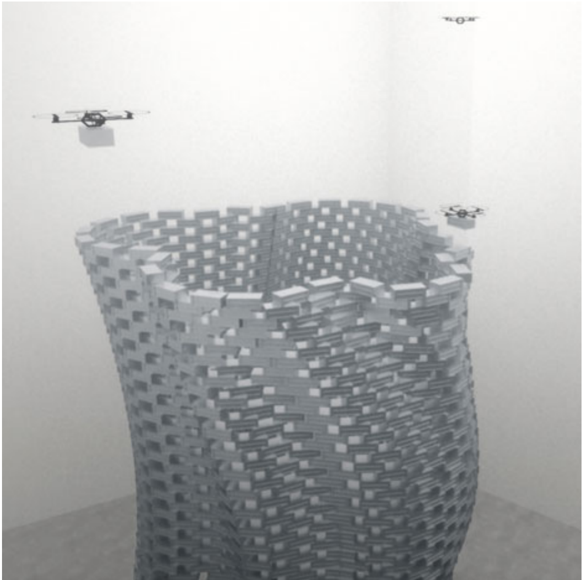
Figure 1-2: An example of a cooperative scheme to build a structure. Each agent has a simple gripper mechanism and the work is distributed among the agents.
