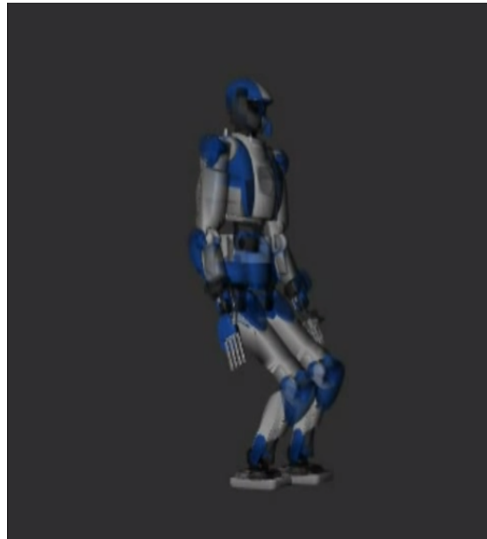
Figure 4.21: Visualization of the walking trajectories using the RViz simulator. Video available at https://www.youtube.com/watch?v=WildzQwH9M0 .
