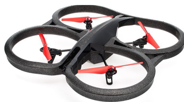
FIGURE 2.2: A quadrotor UAV, Parrot brand.
