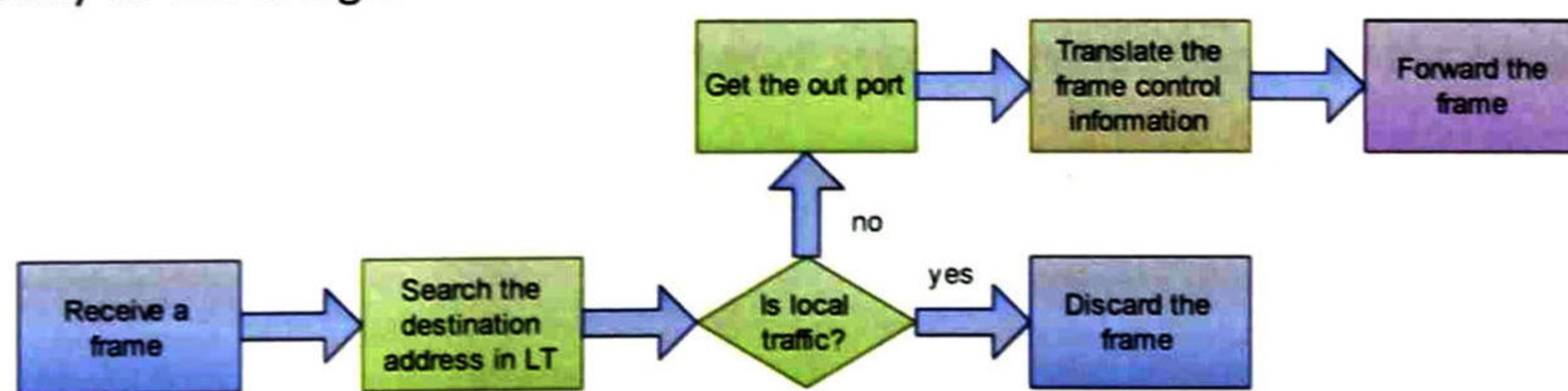
Fig. 13. The general bridging process
