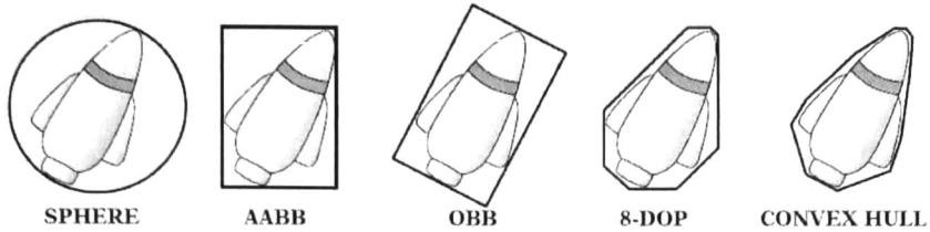
FIGURE 2.2: Type of bounding volumes: Sphere, axis-aligned bounding box (AABB), oriented bounding box (OBB), eight-direction discrete orientation polytope (8-DOP), and convex hull [7].
