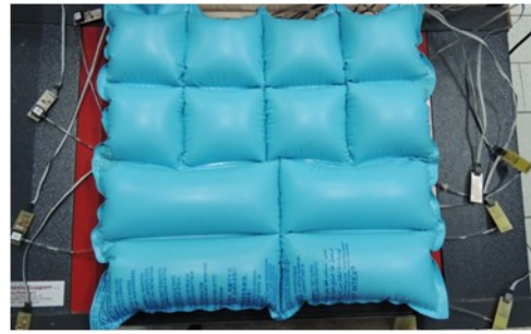
Figure 3. Designed cushion prototype with the sensors connected
