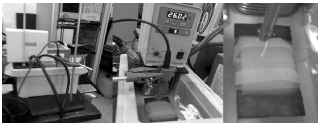
Fig. 1 Experimental setup: assembly of the propagation speed measurement equipment based on the pulse-echo technique.
