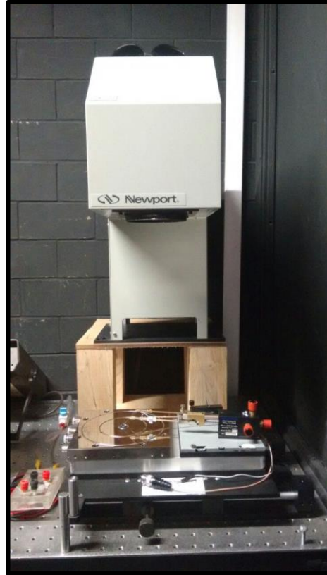
Fig.3.23. Newport 91160 solar simulator.
