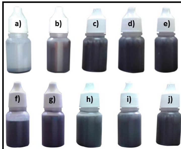
Fig.4.14. The variation in stability of \text{Cu}(\text{In}_{0.7},\text{Ga}_{0.3})\text{Se}_2 ink formulated with EC and Terpeneol, a,b,c,d,e: 40 wt% of Terpeneol with EC wt %-0,1,2,3 and 4 respectively; f,g,h,i,j: 2 wt % of EC with Terpeneol wt% -0,10,20,30 and 40 respectively.
