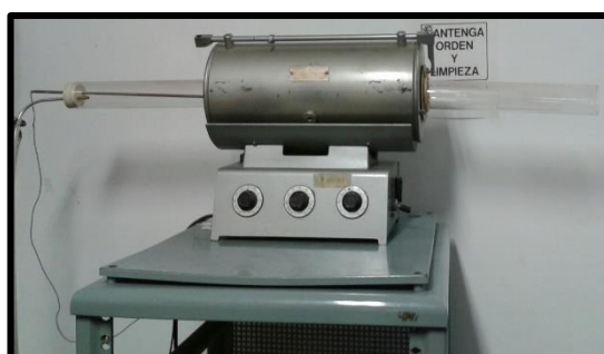
Fig.3.4. Home-made furnace used for air annealing.
