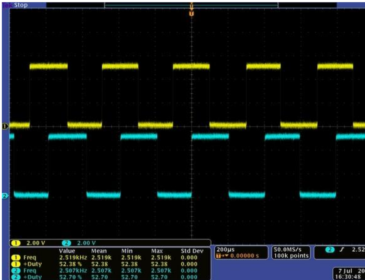
Encoder A and B outputs for 37D mm metal gearmotor with 64 CPR encoder (motor running at 12 V).
