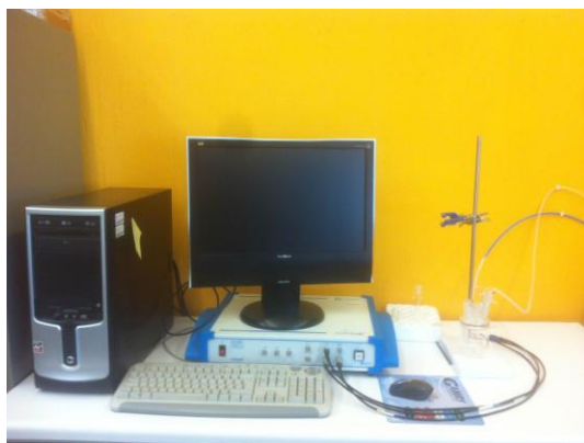
Fig. 3.4. Experimental set-up of the electrochemical cell.
