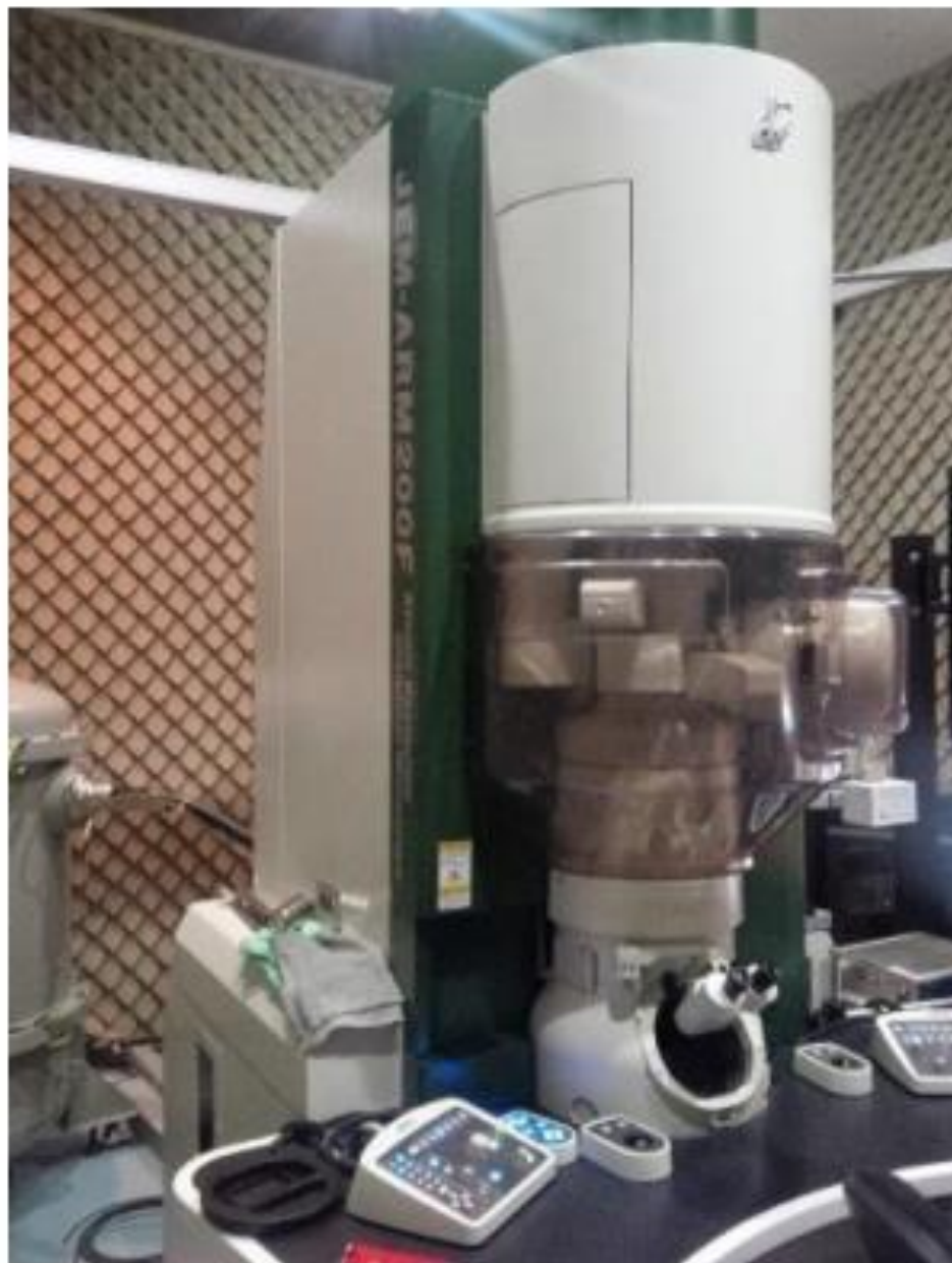
Fig. 3.15. TEM instrument for morphology analysis, EDS and HAADF-STEM techniques.
