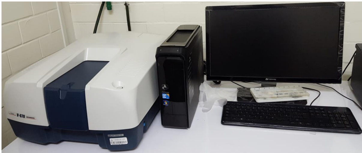
Fig. 3.17. JASCO V-670 UV-VIS-NIR Spectrophotometer.
