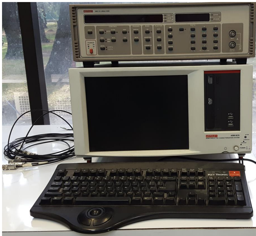
Fig. 3.20. Keithley 4200-SCS semiconductor characterization system.
