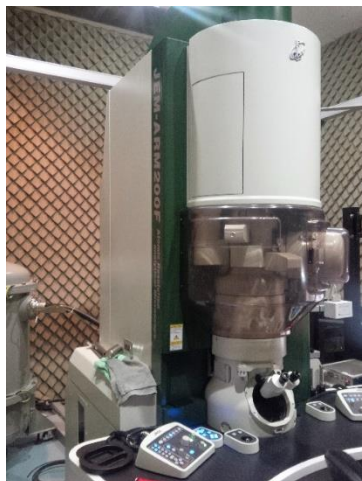
Figure 3.1. TEM instrument for morphology analysis, EDS and HAADF-STEM techniques ( Laboratorio Avanzado de Nanoscopia Electrónica - LANE, CINVESTAV-IPN, Mexico city )
