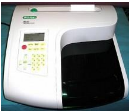
Figure 3.10. Bio-Rad micro plate reader used for MTT assay ( Department of Cell Biology, CINVESTAV-IPN, Mexico city )
