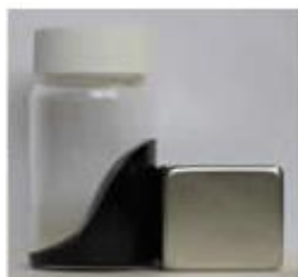
Figure 3.5. As-synthesized black core NPs separated using strong magnet
