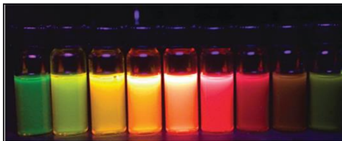
Figure 1.8 CdTe/CdSe QD photoluminescence under UV excitation. The size of the QDs increases from left to right, modulating the emission from 520 nm to the NIR. ( Reproduced with permission from 38 )
