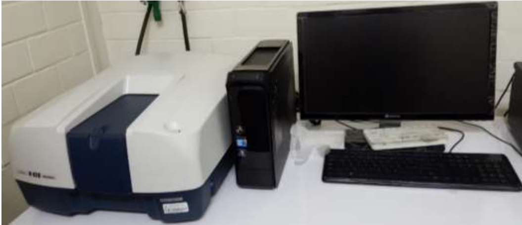
Fig. 3.19. JASCO V-670 UV-VIS-NIR Spectrophotometer.
