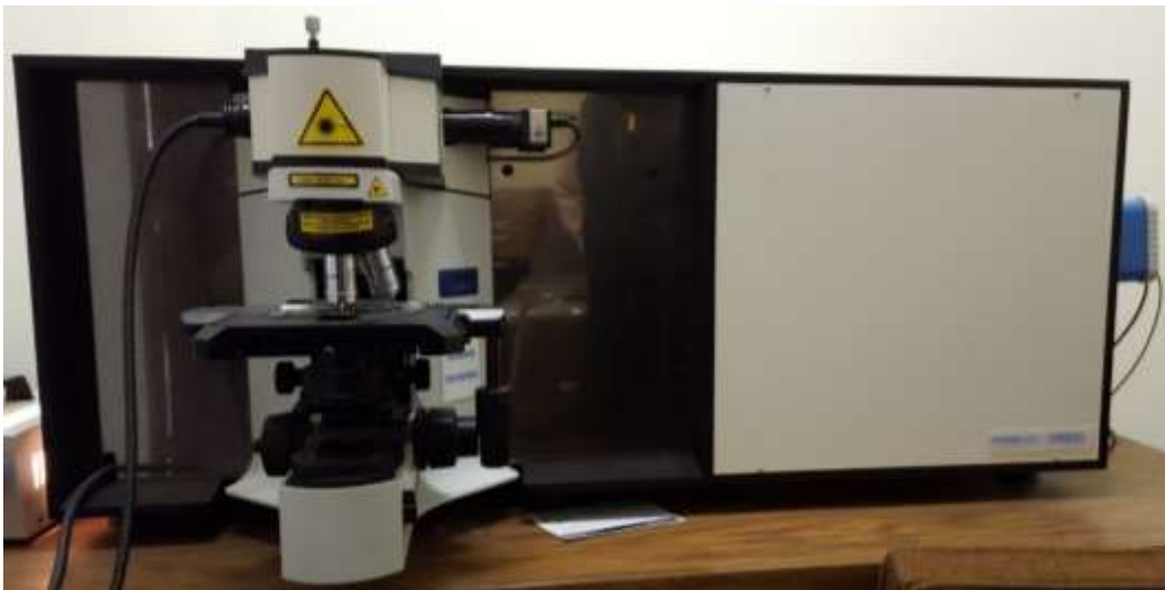
Fig. 3.11. Horiba–Jobin Yvon LabRAM HR800 equipment.
