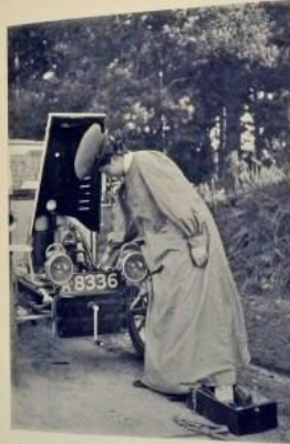
Photo. G. W. Nichols THE ENGINE WILL HEAT RAPIDLY IF YOU FIRST FLOOD THE CARBURETOR HEAVILY.
