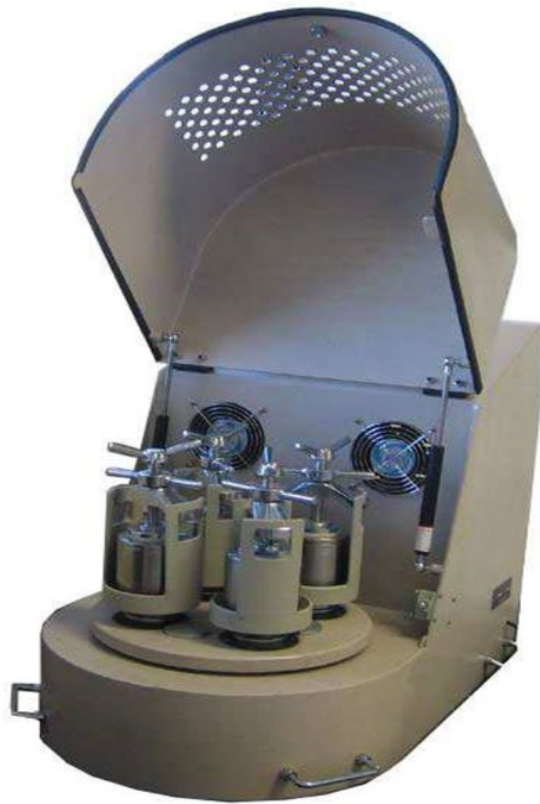
Figura 2.13 Molino Planetario (High Speed Shimmy Ball Mill SFM-1 QM - 3SP2)
