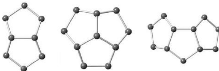
Figure 2.4: Different fused pentagon patterns that can be found in non-IPR isomers. Double fused pentagons (left), triple directly fused pentagons (middle), and triple sequentially fused pentagons (right) (Image taken from ref. [44]).
