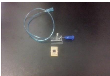
Fig. 4. Microchannel already manufactured with their respective connectors.
