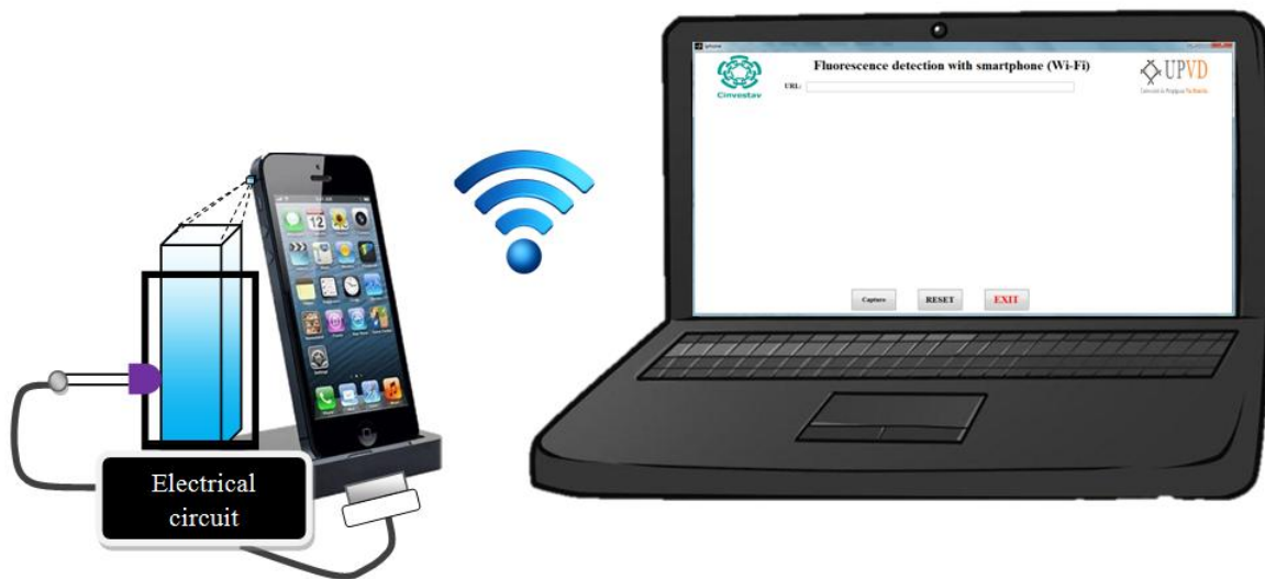
Fig. 30 Fluorescence analyzer developed based on smartphone camera
