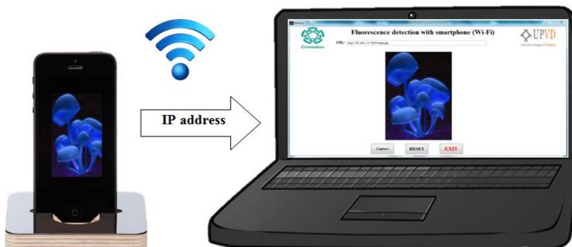
Fig. 31 Interface designed for the fluorescence analyzer based on smartphone camera.
