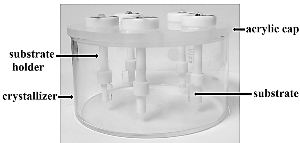
Figure 3.1. Substrates and substrate-holders assembly in the crystallizer containing the bath solution.
