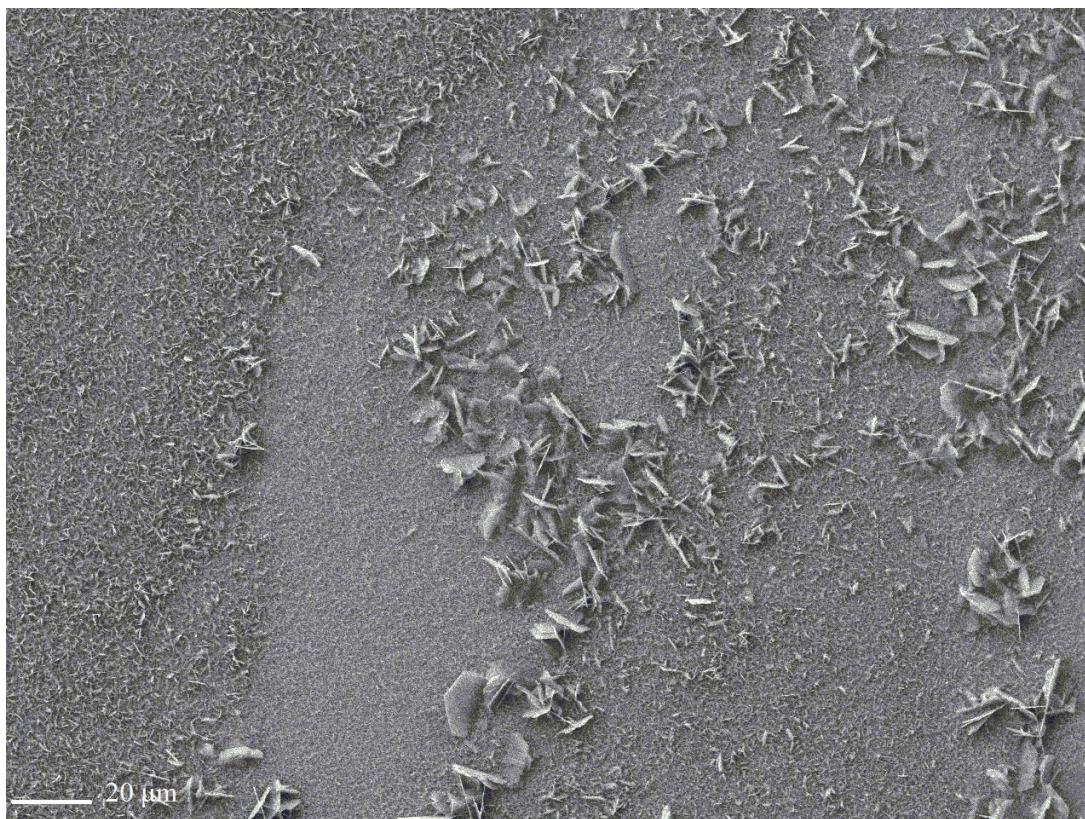
Figure A1.- SEM image for a Simonkolleite film electrodeposited from a 0.1 M \text{Zn}(\text{NO}_3)_2 \cdot 6\text{H}_2\text{O} , 0.1 M KCl aqueous solution at pH= 6.0, 70 °C and the procedure Z1.
