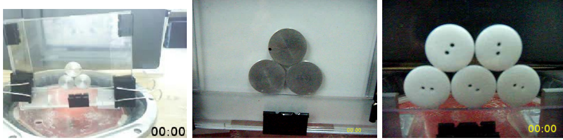
Figure 1.10: Three simple experiments that show sustained rotation under vibration. Left: A minimal 3 disk packing of thin aluminum disks tilted in order to introduce asymmetry. Middle: A minimal 3 disk packing of 1 cm thick steel disks, also tilted. Right: A small packing of plastic buttons. In all three setups disks of the bottom row are fixed.
