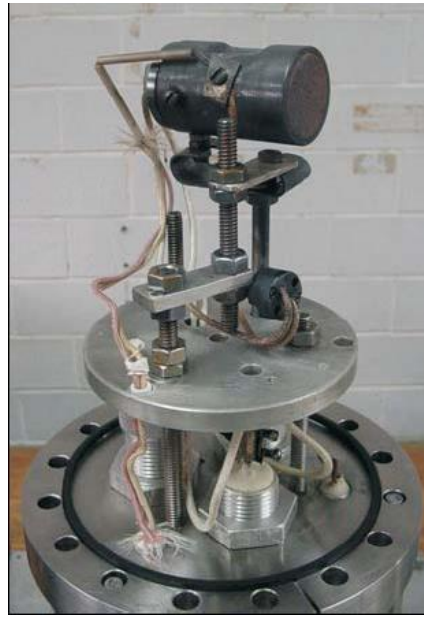
Figure 2.7 Substrate holder and heating system [14].
