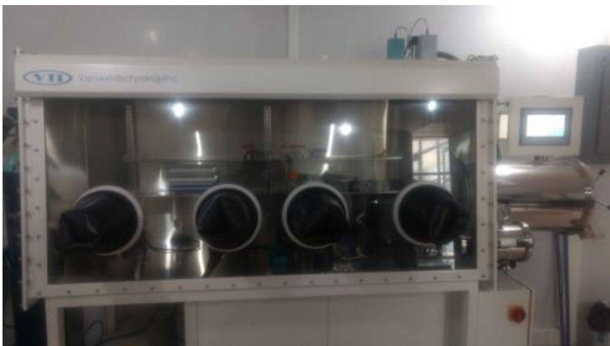
Fig. E-1. The chemical precursors were mixed by grinding inside the glove box shown in the photograph, under a highly pure argon atmosphere.
