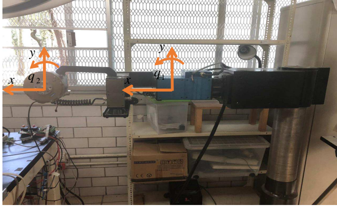
Figura 4.4: Robot planar de 2 GDL
