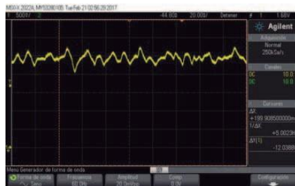
Fig. 5. Long palmar muscle response to a wrist flexion using the dry electrodes wearable system. The signal has a 2.2 Vdc offset in order to send it by the analog input to the microcontroller.
