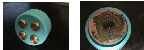
Fig. 8. Final stage of the electrodes integrated to the sEMG signal acquisition sytem.
