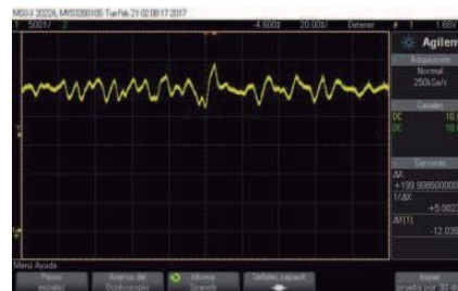
Fig. 7. Long palmar muscle response to a wrist flexion using Ag/AgCl wet electrodes wearable system. The signal has a 2.2 Vdc offset in order to send it by the analog input to the microcontroller.
