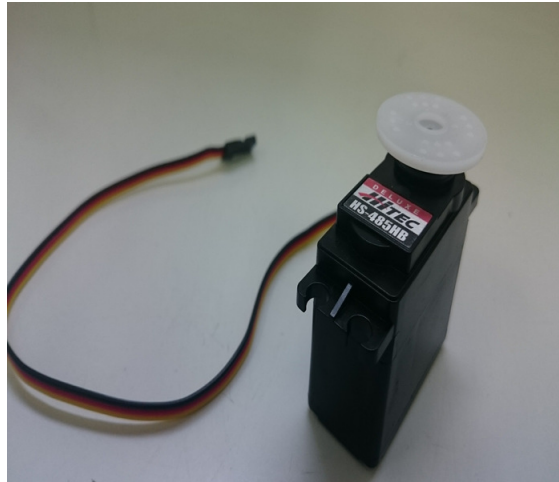
Figura 4.3: Servomotor de RC HS-485HB.
