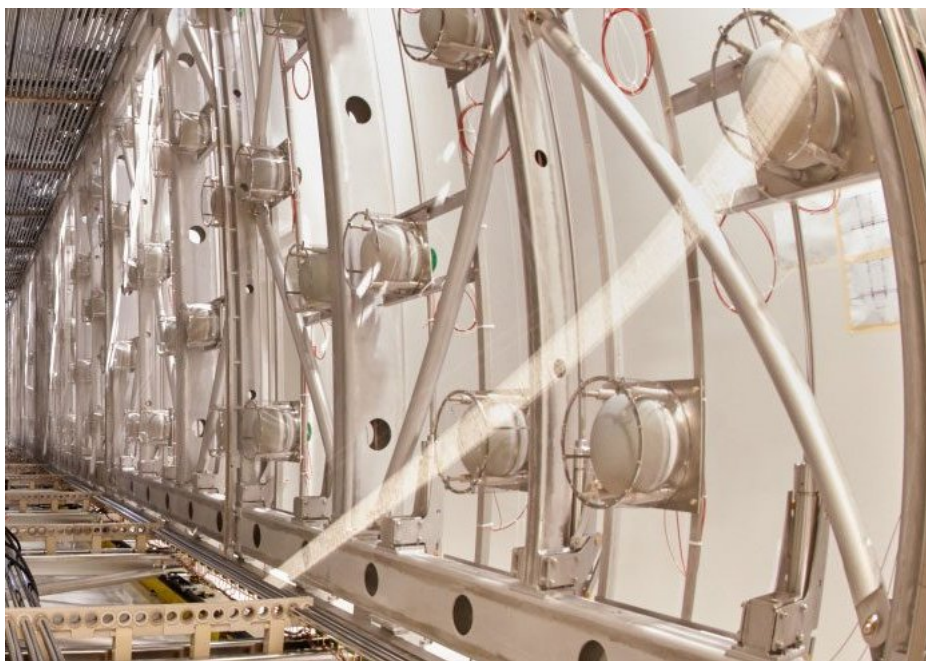
Figure 4.9: PMTs placed in one of the ICARUS TPCs. Image from: https://icarus.fnal.gov/ .
