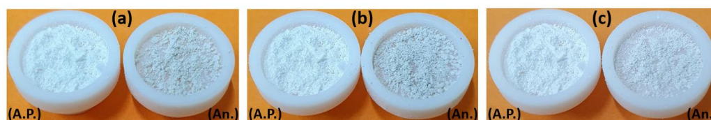
Figure 3.1.9.3. Powder of the (a) bar-, (b) cube-, and (c) flower-like morphologies before (as-prepared – A.P.) and after the three-step thermal treatment; (1) 120 °C for 3 h, (2) 200 °C for 2 h, and (3) 250 °C for 16 h (An.).
