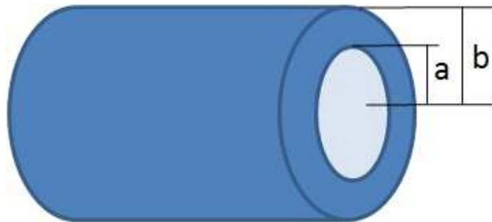
Figure 3.1: Cylindrical waveguide corresponding to a circular cross-section. The core (inner) radius is of length= a , while the clad (outer) radius is of length = b .
