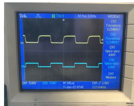
(b) Response of the left limb optocoupler circuit to a square signal
