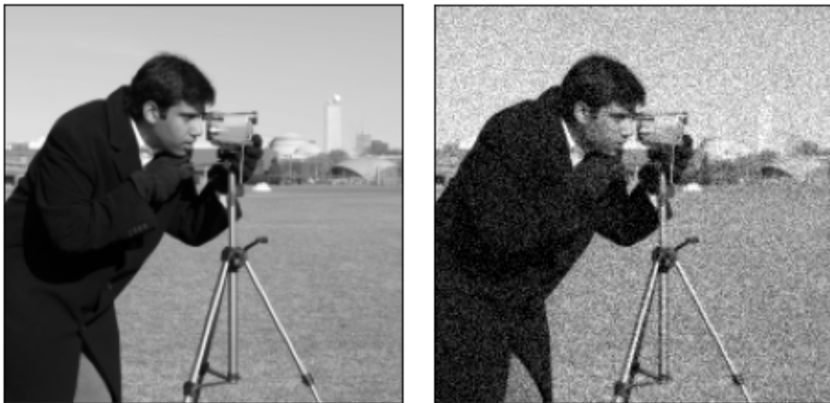
Figure 4.4: Left side, the original image. Right side, the image plus Gaussian noise, mean zero and variance 0.05.
