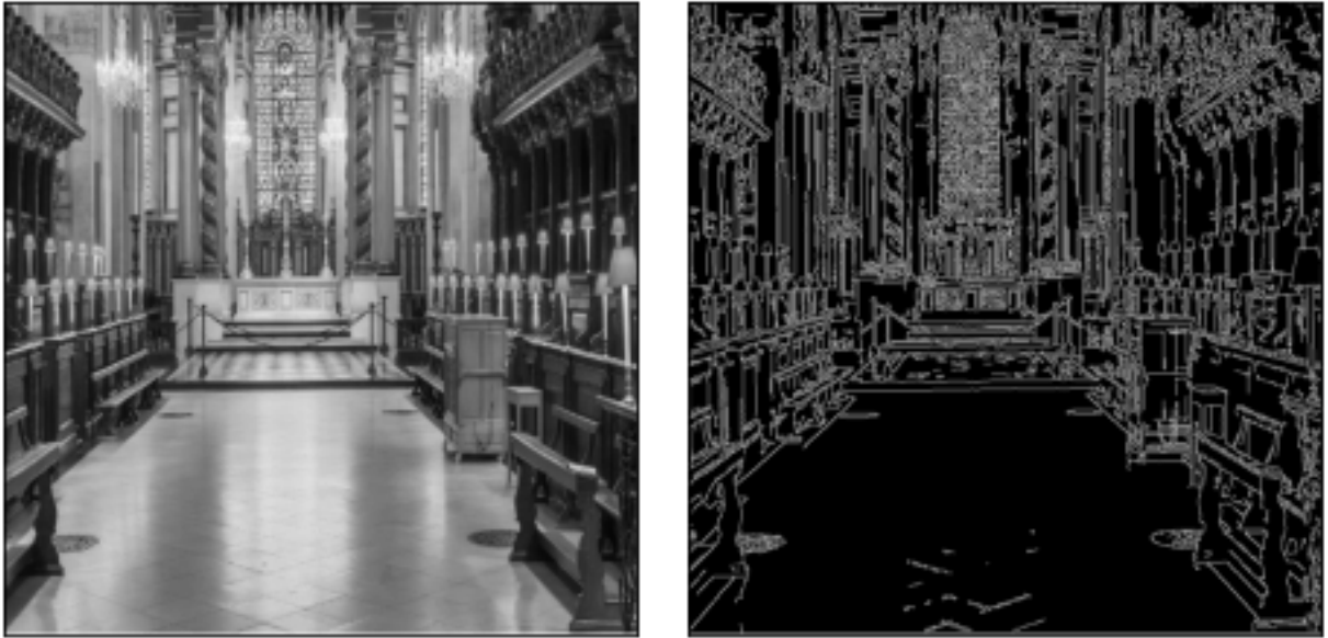
Figure 4.1: Left side, the original image. Right side, edges obtained by using a Canny edge detector. See Section B.1
