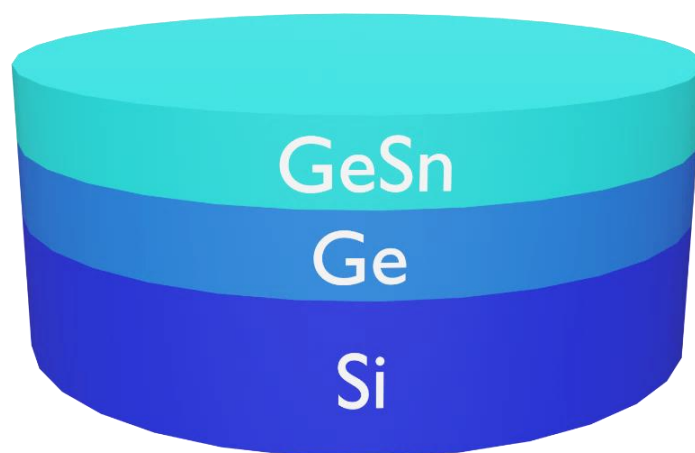
Fig. 6 GeSn thin film grown over a Ge buffer on a Si substrate
