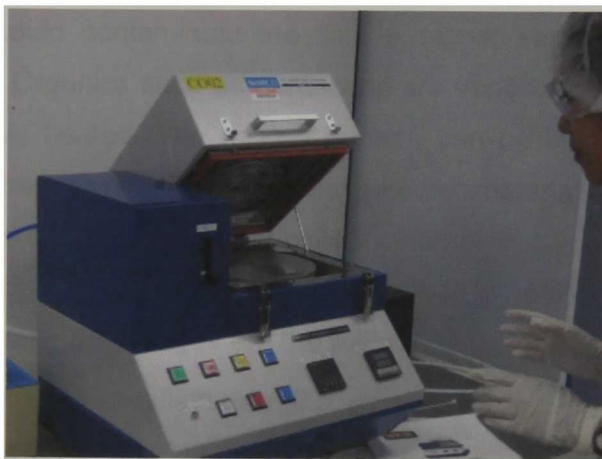
Figure 2.3 UV-Ozone cleaning. The equipment employed was Samco UV-Ozone Stripper/Cleaner model UV-1.
