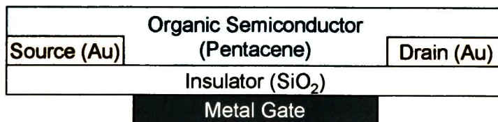
Figure 1.1 Schematic representation of an OTFT. The electrodes (the source and the drain) are made from a metal, typically Au. Pentacene is becoming the organic "semiconductor" of choice. SiO_2 is commonly employed for the insulating layer.
