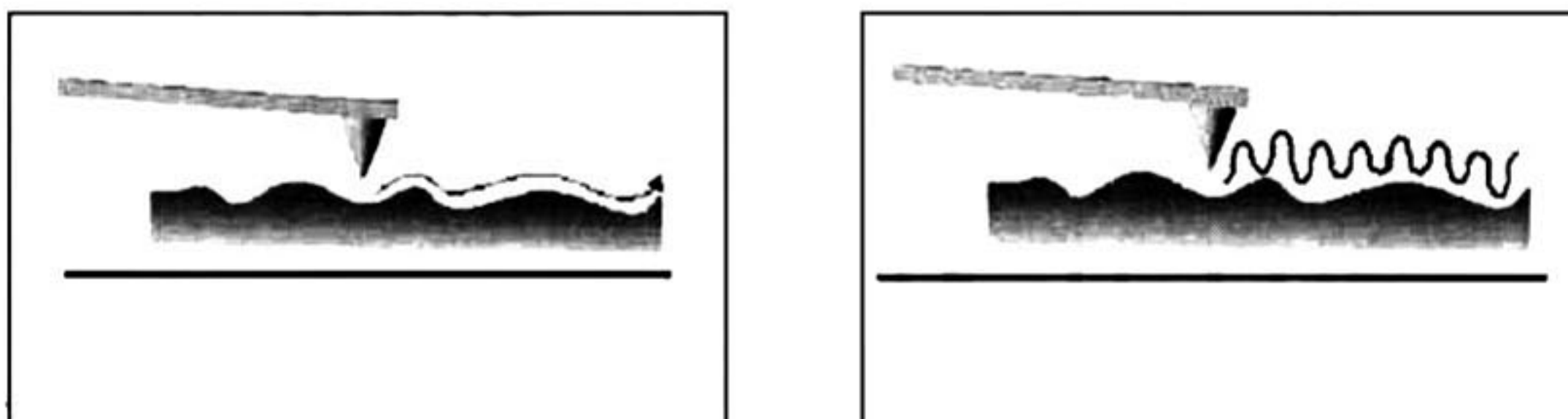
Figure 3.7 (a) In contact mode AFM the probe directly follows the topography of the surface as it is scanned. (b) In vibrating mode, changes in probes vibrations are monitored to establish the force of the probe onto the surface.
